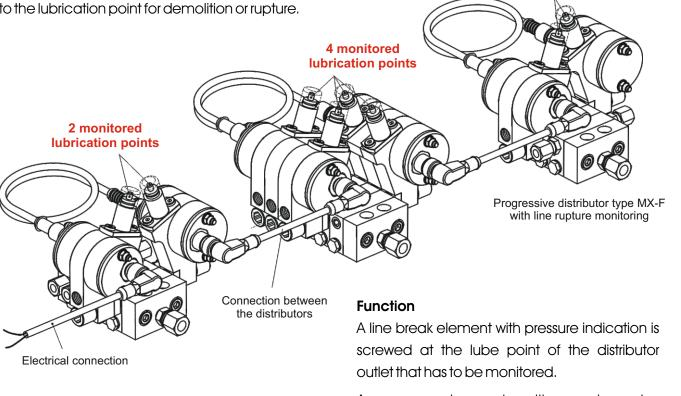
A pressure makeup valve with non-return valve is screwed directly into the lube point. If pressure is reduced due to line break, the pin of the pressure indication becomes invisible and the electrical circuit is interrupted.
